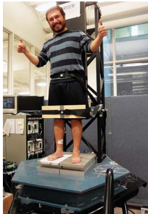
The author rides the Riser at Caris Lab. The device can be used to tilt subjects while varying the angle of the platform surface on which the subject stands, for use in medical research and rehab.
